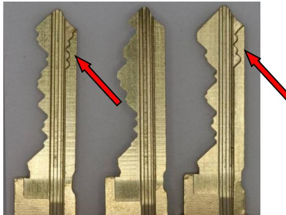
**Picture 19: Level 1 (middle) and level 2 tips of the ASSA d12 keys (red arrows)**
