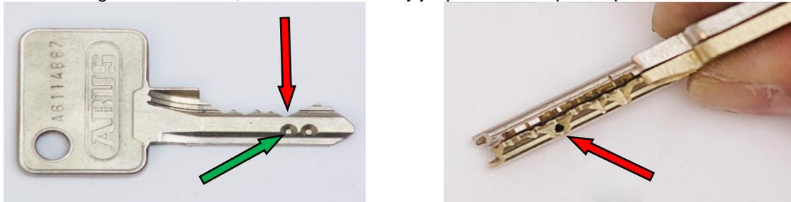
**Picture 53a and 53b: Abus TS5000 key with deep cut**
