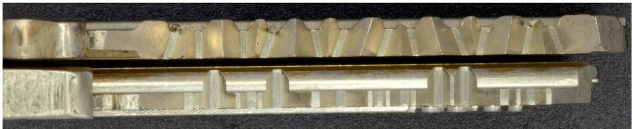
**Picture 15: Top view of Medeco GMK key (top) and ASSA d12 (bottom)**
