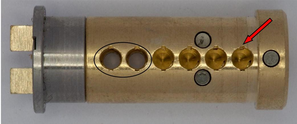
**Picture 25: The plug without pins**
