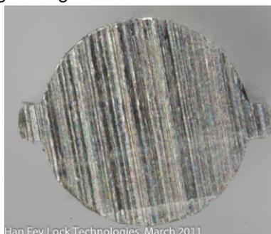
**Picture 22: View on the raw material of the pins**
