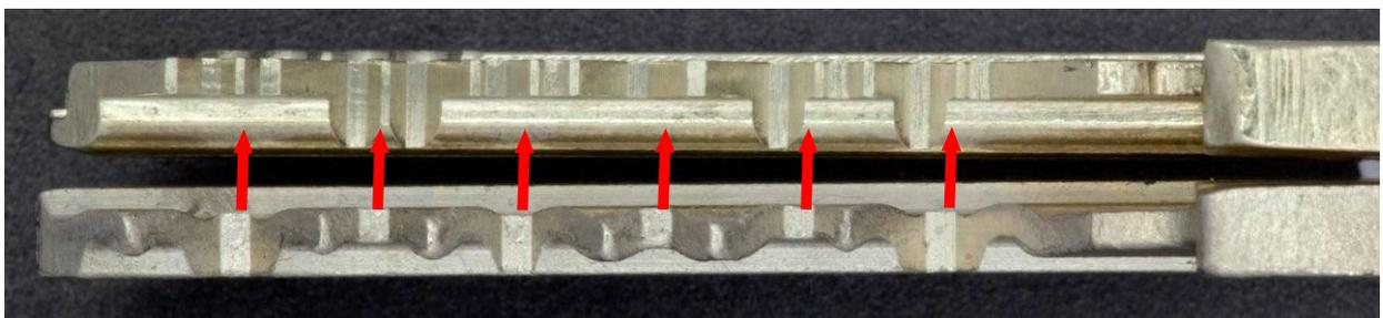
**Picture 16: Keycuts distance between ASSA 600 (bottom) and ASSA d12 (top)**
