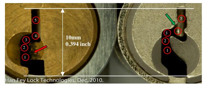
*Picture 54: Detailed picture of ASSA d12 keyway and Abus TS5000 keyway Note: The circles all have the same diameter, this to show the possible space in the keyway. Note: Some dirt / oil get in the ribs of the key. When you insert the key then in the lock, the ribs in the keyway will clean the key. You can see the dirt on the ribs (red arrow).*
