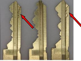
Picture 19: Level 1 (middle) and level 2 tips of the ASSA d12 keys (red arrows)
