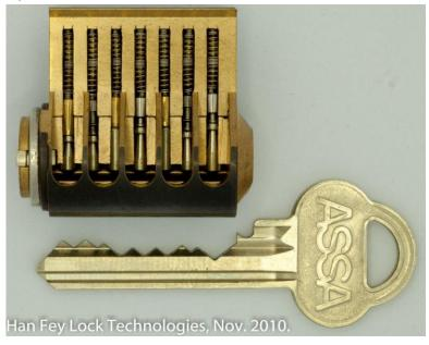
Picture 6: ASSA 700 cutaway in locked position
