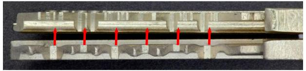
*Picture 16: Keycuts distance between ASSA 600 (bottom) and ASSA d12 (top) Note: I did not line up the keys exactly.*
