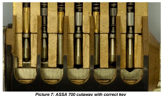
Note: In this cutaway you can see clearly how the bottom pins fit in the cuts in the key, really a marvellous cutaway.
