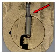
Picture 37a and 37b: Plug in locked position and tilting top pin in the housing
