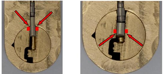
**Picture 35a and 35b: A high lifted pin and a short pin.** Note: The red squares are the right and the left wing on the bottom pin Note: The red arrows mark the positions were the bottom pin rests on the wings. Note: The rotation of the plug is slightly turned, because of the play in the diameters
