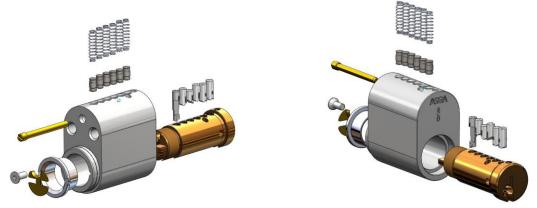
Picture 9: Exploded view of the ASSA d12
