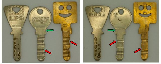
*Picture 56a and 56b: Left and right side of the impressioned Lips Keso keys* Note: The green arrow marks the "bottom" of the key. In the picture of the padlock you can see the red mark on the side of the key. People who do impressioning do know why. Note: The original Lips Octro key is not the key from the padlock. It is just a random key out of my collection.
