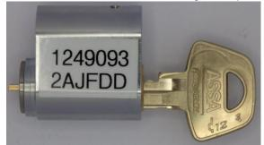
Picture 20: The level 1 key does not go all the way into a level 2 cylinder
