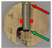
*Picture 36a, 36b and 36c: Different "shielding" positions of the bottom pins Note: The red squares are the right and the left wing on the bottom pin Note: The height and position of these wings can vary*
