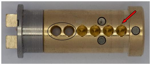
Picture 25: The plug without pins
