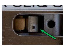
Picture 2a,2b and 2c: Padlock with cover plate & without + Detail of the cam in the locked position
