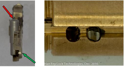
*Picture 24a and 24b: The longer bottom pins with the key.* Note: On the left picture you can see the tip of the key (green arrow), with the longer bottom pin (red arrow)
