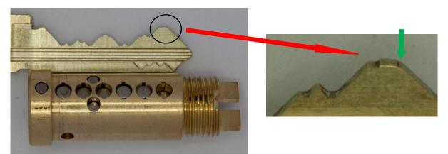
*Picture 26a and 26b: Pins in the plug in the locking position and detail of the tip Note: The pins do not rest on the bottom of the chamber. Reason to look further.*
